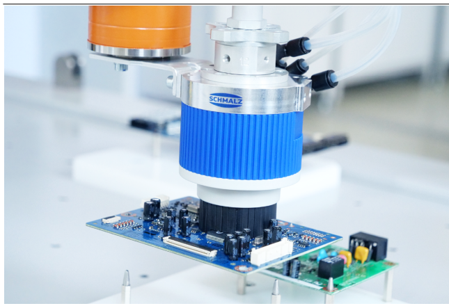
Flow grippers SCG-HSS for handling assembled printed circuit boards
